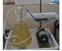
Fig. 2: Experimental Setup of Side Stream Membrane Bioreactor (SSMBR)
